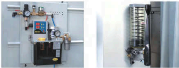
Grease supply unit in simple design provide appropriate lubrication quantity at linear guide ways, ball-screw that ensures machinery service life (CNC 3).
