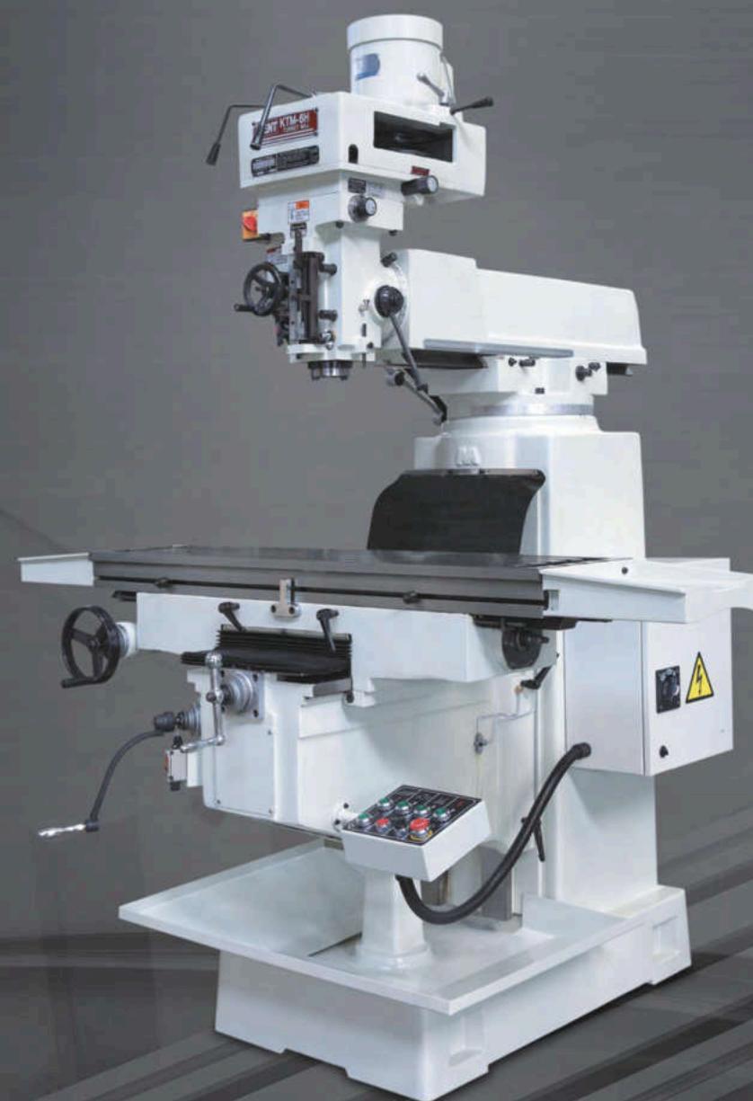
KTM-6H 1370 X 330mm (Dimension of work table) X/Y/Z 830X330X420
